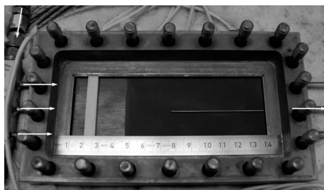
Fig. 2. Picture of the opened channel reactor with the catalyst plate installed, the flow straightener, and the movable sampling capillary.
